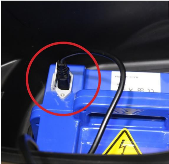
7. Connect the IEC C13 connector from the charger to the battery, we need to lift the top that cover the connection in the battery.
