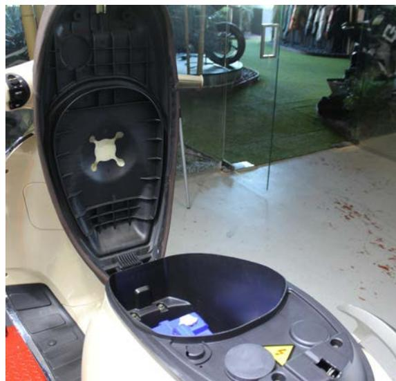
3. Lift up the seat to Access to the battery connections.
