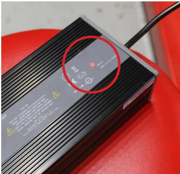
8. Wait a few seconds and check out that the LED indicator of the charger is on with RED light.
