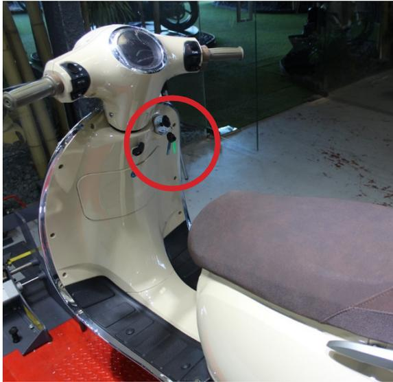
1. To access to the battery, it will be necessary put the key inside the start lock.
