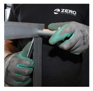
5. Set the two wrenches in both sides of the screw to remove it. One at the inner part and the other on the exterior.
