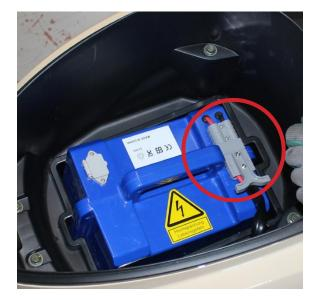
20. Connect the battery to the exact connector to check if its functioning is correct.
