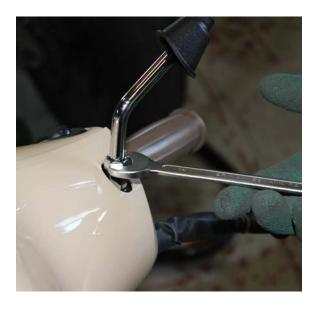
18. Screw it by using a 14mm wrench.
