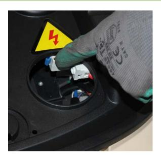
21. Turn on the kill-switch to allow current in the circuit.
