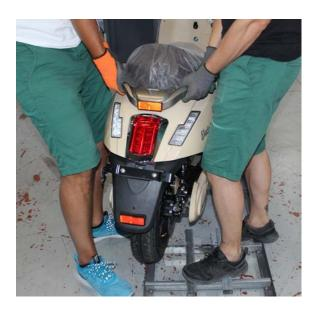
12. Once we have removed the tapes, lift the motorbike by holding it and move it to one side, out of the structure.
