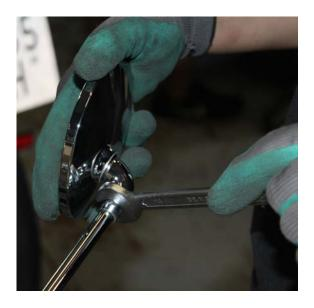
19. Put the mirrors in the correct position and softly screw it with the 14mm wrench.
